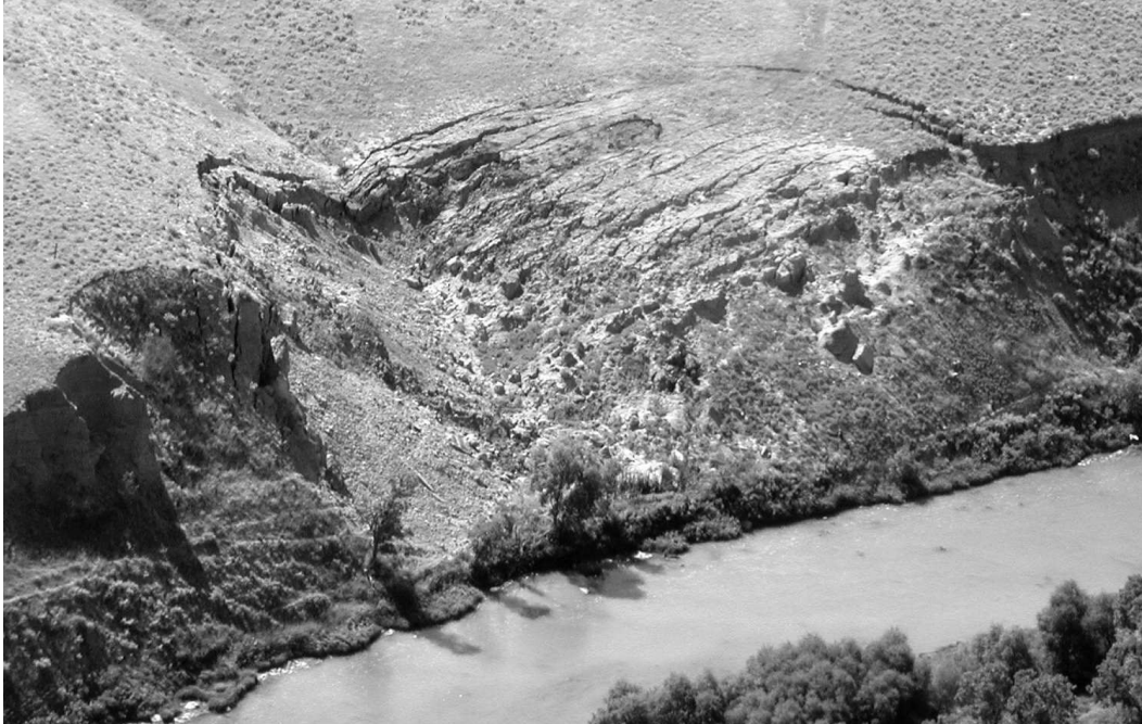
Figure 1. Natural coal bed fire along bank of Tongue River north of Sheridan, Wyoming. Note concentric fissures created by collapse of coal bed. Photo courtesy of Gerald Queen, BLM Buffalo Field Office.
